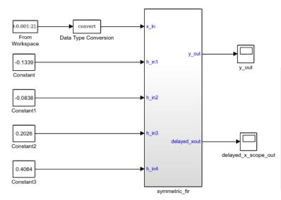
This example shows how to use HDL Coder to check, generate, and verify HDL for a fixed-point symmetric FIR filter. In MATLAB, type the following: checkhdl('sfir\_fixed/symmetric\_fir') makehdl('sfir\_fixed/symmetric\_fir') makehdltb('sfir\_fixed/symmetric\_fir') Or double-click the blue button at the bottom to see the dialog.
