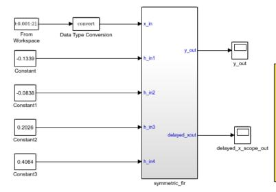
This example shows how to use HDL Coder to check, generate, and verify HDL for a fixed-point symmetric FIR filter. In MATLAB, type the following: checkhdl('sfir\_fixed/symmetric\_fir') makehdl('sfir\_fixed/symmetric\_fir') or double-click the blue button at the bottom to see the dialog.
