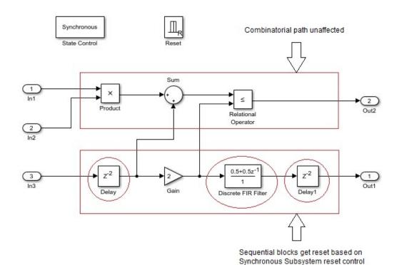
The reset port in the Resettable Synchronous Subsystem block adds reset capability to blocks inside the subsystem that have state. This includes blocks that need not have an external reset port capability, such as filters, Stateflow Chart, and MATLAB Function blocks. For HDL code generation, the **Reset trigger type** of the Reset port is set to level hold by default.
