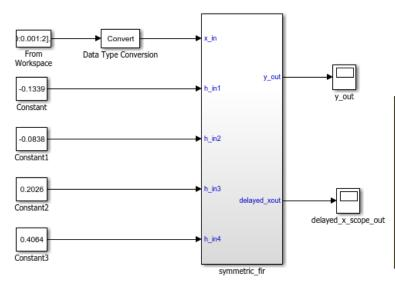
This example shows how to use HDL Coder to check, generate, and verify HDL for a fixed-point symmetric FIR filter. In MATLAB, type the following: checkhdl('sfir\_fixed/symmetric\_fir') makehdl('sfir\_fixed/symmetric\_fir') or double-click the blue button at the bottom to see the dialog.
